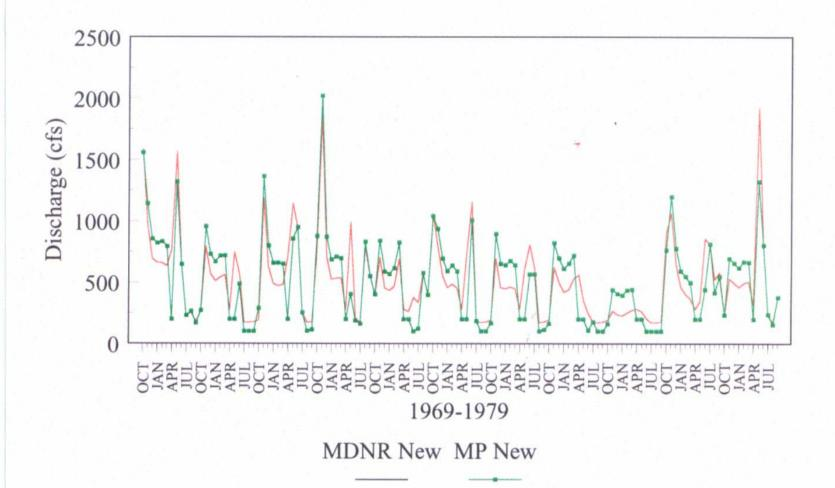
Figure 22. Comparison of Cloquet River flows resulting from operating schemes proposed by MP and MDNR for the reservoirs.
