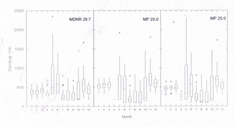
Figure 4. Box - whisker plots of monthly outflows from Island Lake reservoir under operating schemes proposed by MP and MDNR.
