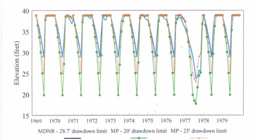
Figure 6. Comparison of Island Lake reservoir elevations resulting from operating schemes proposed by MP and MDNR. Results are produced from reservoir model developed by BEAK using hydrologic inflow data for water years 1969 through 1979. MP proposes operating Island Lake with drawdowns to 20 or 25 feet elevation. For testing, we assumed continuous operation under each drawdown limit. Results are displayed by water year, that starts with October and ends in the September of the named year.
