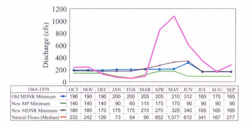
Figure 1. Recommended minimum outflows for Island Lake Reservoir proposed by Minnesota Power (MP) and the Minnesota Department of Natural Resources (MDNR). Median flows are presented to show the relationship (timing, magnitude) of each proposal to natural conditions. Median flows were developed by the MDNR, Division of Waters and represent natural flows without the effect of the reservoirs.
