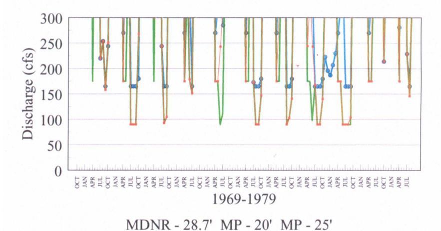
Figure 3. Close-up of outflows from Island Lake Reservoir using a smaller scale to show the timing and magnitude of minimum flows for proposals by MP and MDNR, 1969 to 1979.
