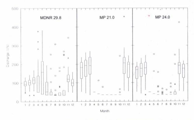
Figure 30. Box - whisker plots of monthly outflows from Whiteface reservoir under operating schemes proposed by MP and MDNR.
