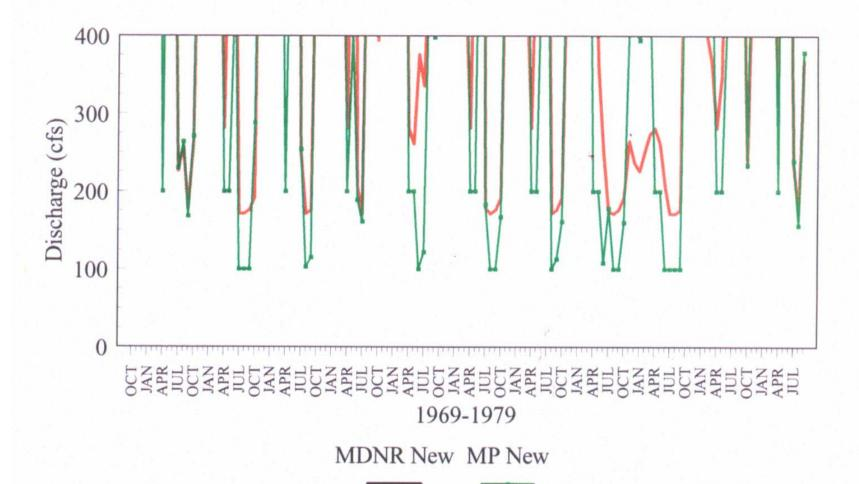
Figure 23. Close-up of flows in the Cloquet River using a smaller scale to show the timing and magnitude of minimum flows for proposals by MP and MDNR, 1969 to 1979.
