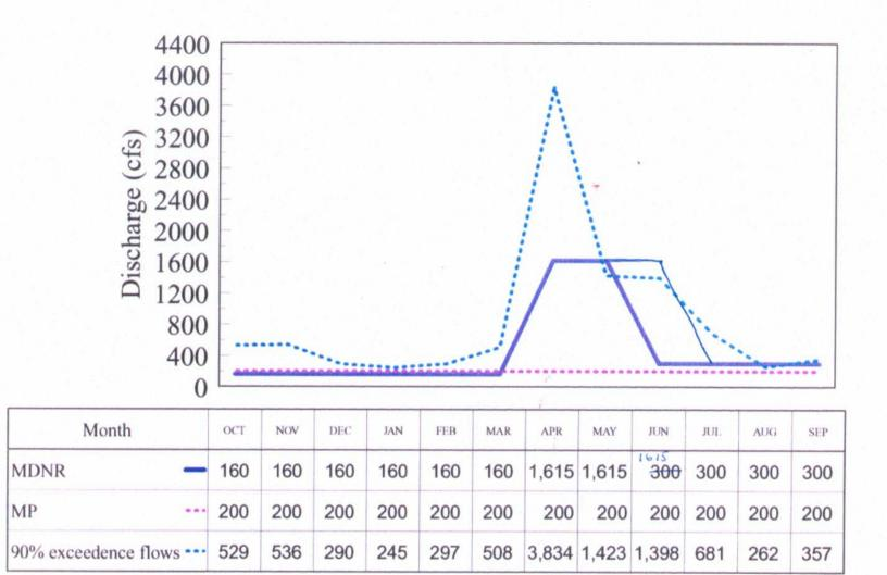
Figure 32. Recommended minimum outflows proposed by MP and the MDNR for the bypassed reach below Fond Du Lac Reservoir and 90% exceedence flows (low flows). Low flows are presented to show the relationship (timing, magnitude) of each proposal to natural conditions. MP will also provide water that cannot be used by the turbines (> 2000 cfs).
