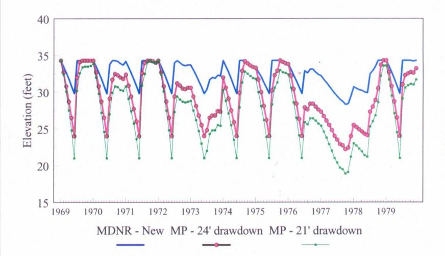
Figure 25. Comparison of Whiteface Reservoir elevations resulting from operating schemes proposed by MP and MDNR. Elevations are produced from the reservoir model developed by BEAK, and use the minimum outflow recommendations, maximum drawdown elevations of each proposal (MP - 21, 24 feet, MDNR - 29.8 feet), and the hydrologic inflow data for water years 1969 through 1979. Results are displayed by water year, that starts with October and ends in the September of the named year.
