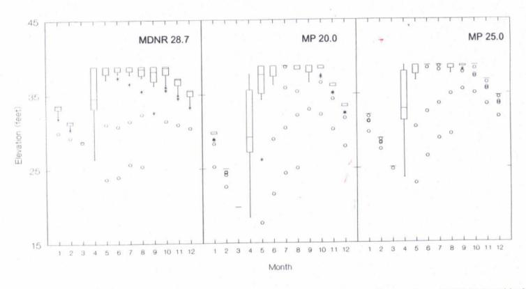
Figure 9. Box-whisker plots of monthly elevations from Island Lake Reservoir under operating schemes proposed by MP and MDNR.
