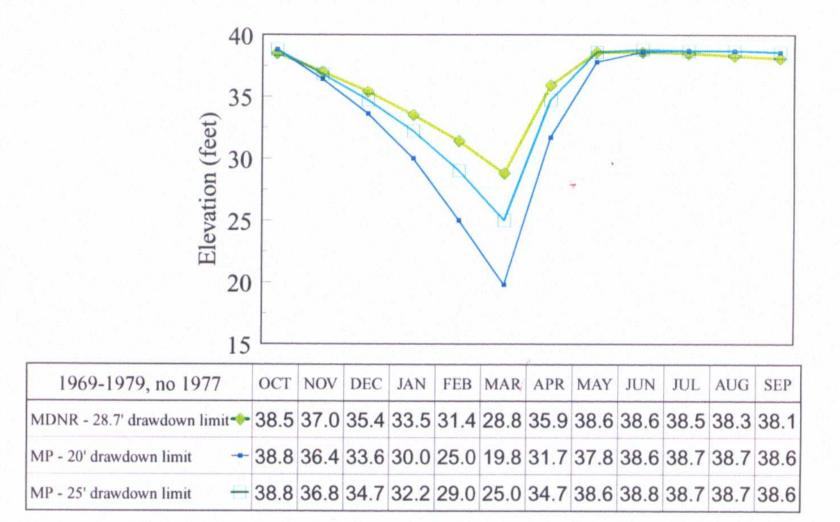
Figure 8. Average monthly elevations of Island Lake Reservoir for operating schemes proposed by MP and MDNR. Results are produced from the reservoir model developed by BEAK using hydrologic inflow data for water years 1969 through 1979, without the 1977 drought year. Water year 1977 was not included in the calculation of average monthly elevations to produce numbers typical of normal operations.
