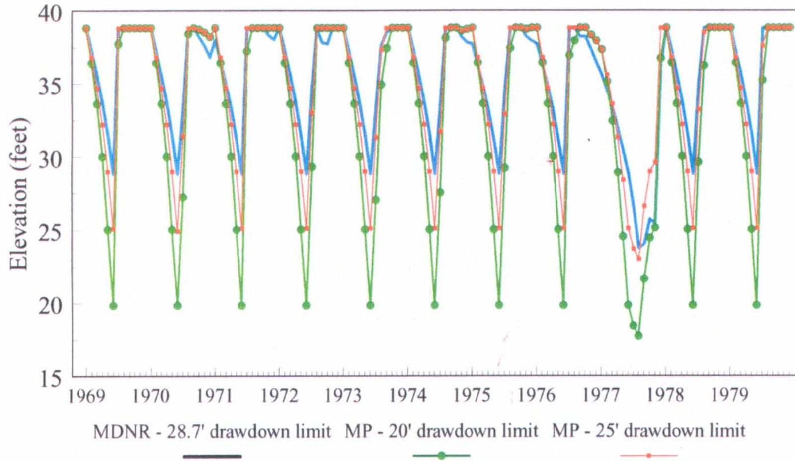
Figure 6. Comparison of Island Lake reservoir elevations resulting from operating schemes proposed by MP and MDNR. Results are produced from reservoir model developed by BEAK using hydrologic inflow data for water years 1969 through 1979. MP proposes operating Island Lake with drawdowns to 20 or 25 feet elevation. For testing, we assumed continuous operation under each drawdown limit. Results are displayed by water year, that starts with October and ends in the September of the named year.
