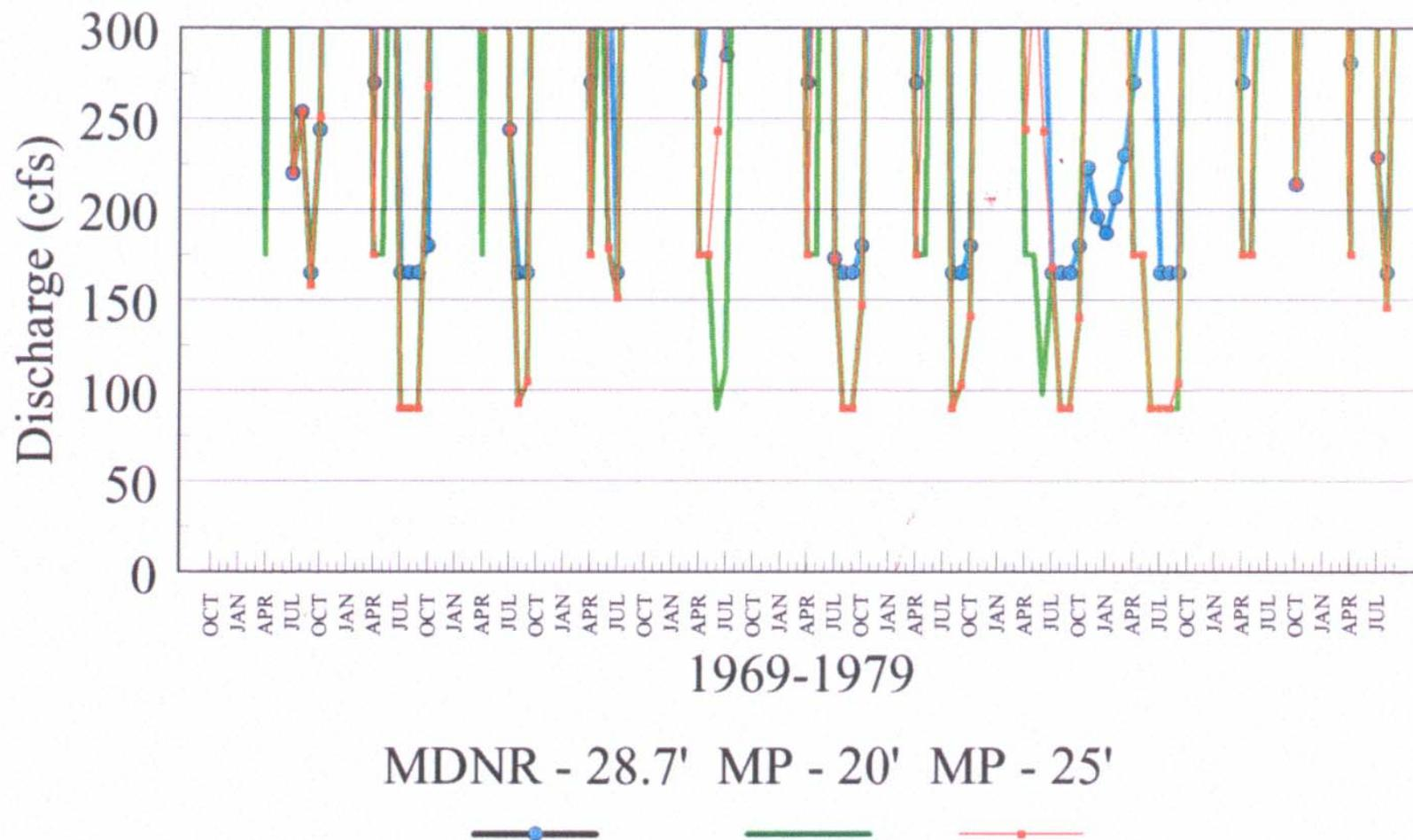
Figure 3. Close-up of outflows from Island Lake Reservoir using a smaller scale to show the timing and magnitude of minimum flows for proposals by MP and MDNR, 1969 to 1979.
