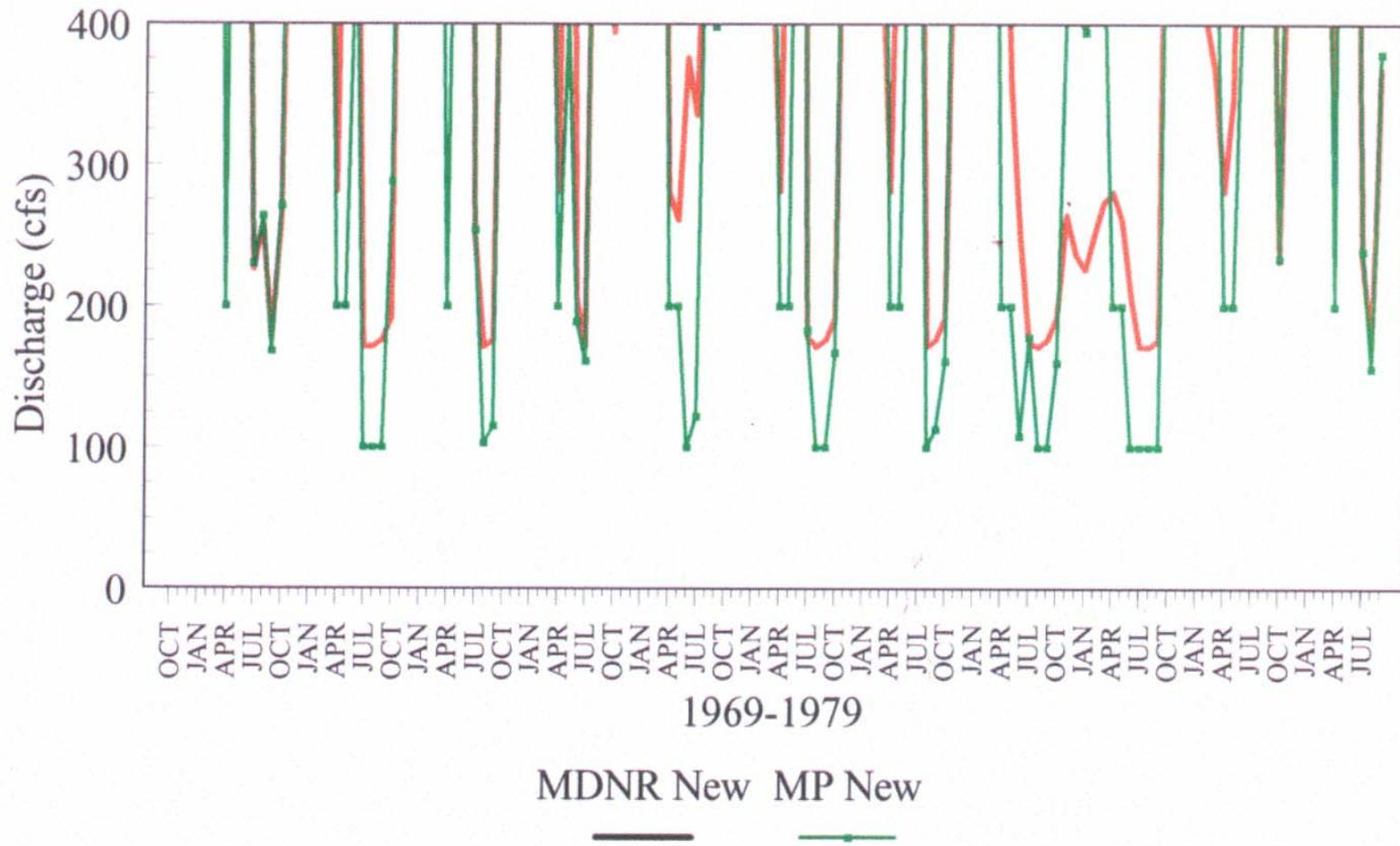
Figure 23. Close-up of flows in the Cloquet River using a smaller scale to show the timing and magnitude of minimum flows for proposals by MP and MDNR, 1969 to 1979.
