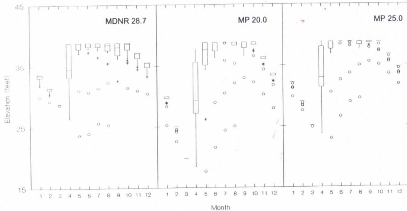
Figure 9. Box-whisker plots of monthly elevations from Island Lake Reservoir under operating schemes proposed by MP and MDNR. Outflows are produced from the reservoir model developed by BEAK, and use the minimum outflow recommendations, maximum drawdown elevations of each proposal (MP - 20, 25 feet, MDNR - 28.7 feet), and the hydrologic inflow data for water years 1969 through 1979.
