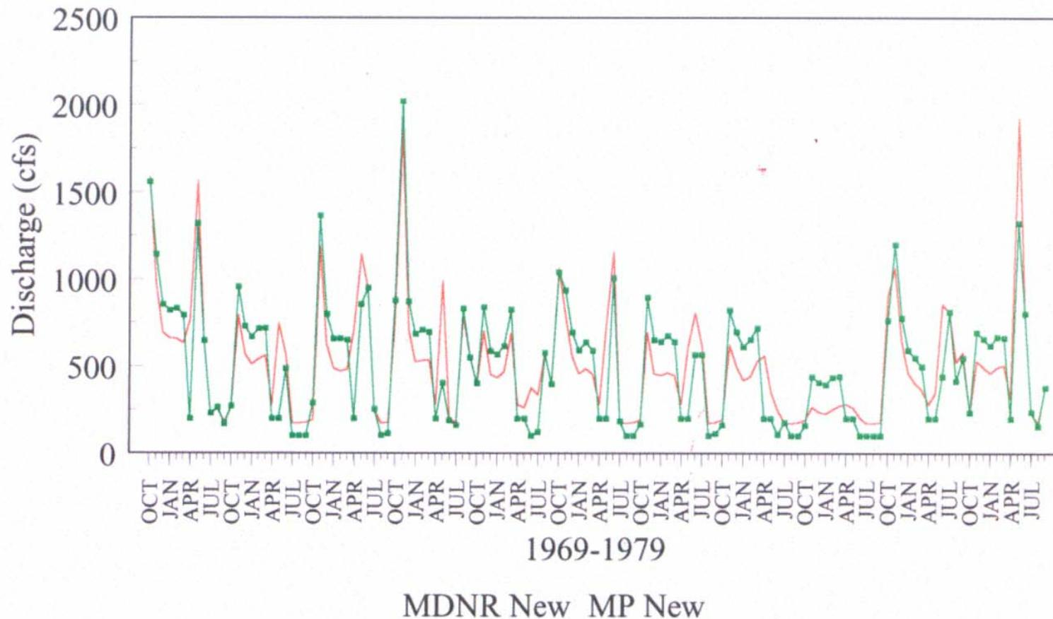
Figure 22. Comparison of Cloquet River flows resulting from operating schemes proposed by MP and MDNR for the reservoirs. Outflows are produced from the reservoir model developed by BEAK, and use the minimum outflow recommendations for each reservoir, maximum drawdown elevations of each proposal, and the hydrologic inflow data for water years 1969 through 1979. Results are displayed by water year, that starts with October and ends in the September of the named year.
