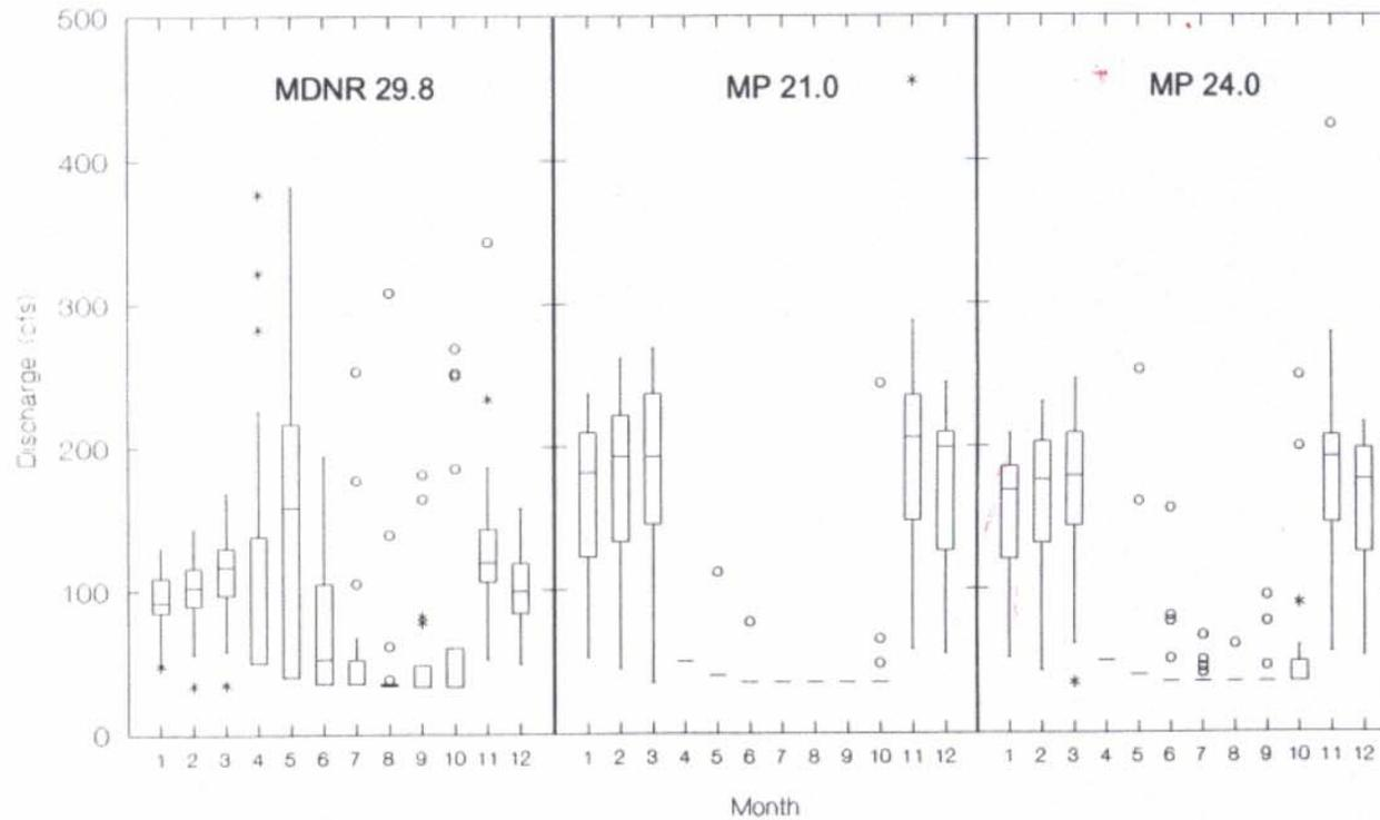
Figure 30. Box - whisker plots of monthly outflows from Whiteface reservoir under operating schemes proposed by MP and MDNR. Outflows are produced from the reservoir model developed by BEAK, and use the minimum outflow recommendations, maximum drawdown elevation of each proposal (MP - 21 and 24 feet, MDNR - 29.8feet), and the hydrologic inflow data for water years 1969 though 1979.
