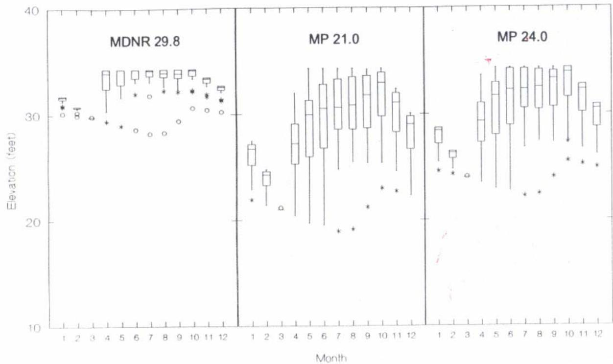
Figure 27. Box - whisker plots of monthly elevations of Whiteface reservoir under operating schemes proposed by MP and MDNR. Elevations are produced from the reservoir model developed by BEAK, and use the minimum outflow recommendations, maximum drawdown elevation of each proposal (MP - 21 and 24 feet, MDNR - 29.8 feet), and the hydrologic inflow data for water years 1969 through 1979.
