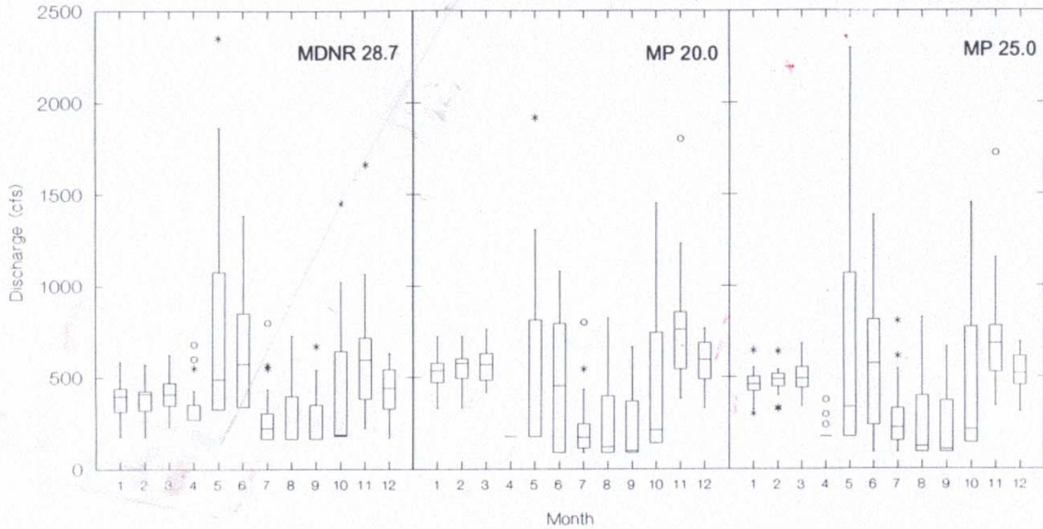
Figure 4. Box - whisker plots of monthly outflows from Island Lake reservoir under operating schemes proposed by MP and MDNR. Outflows are produced from the reservoir model developed by BEAK, and use the minimum outflow recommendations, maximum drawdown elevation of each proposal (MP - 20 and 25 feet, MDNR - 28.7feet), and the hydrologic inflow data for water years 1969 though 1979.
