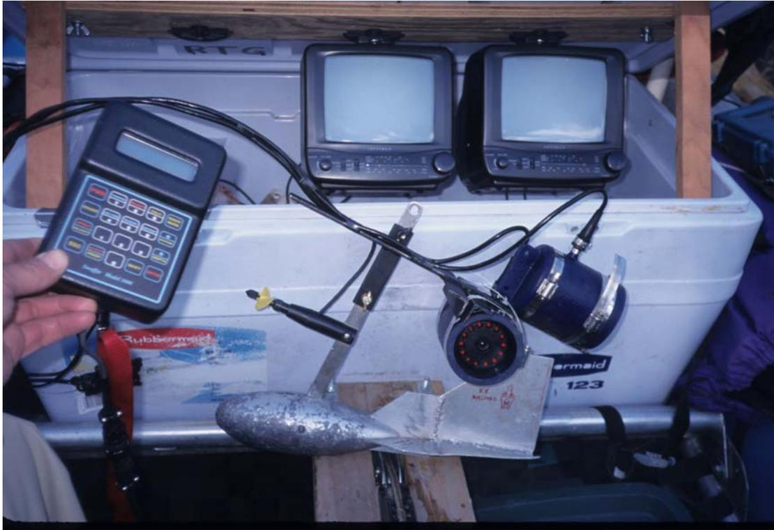
Figure 4. Underwater Fish Eye videography cameras, direct current black and white video monitors, Swoffer water velocity meter, and down-rigger bomb used to search deepwater during the Klamath River habitat suitability investigation, 1999-2000.
