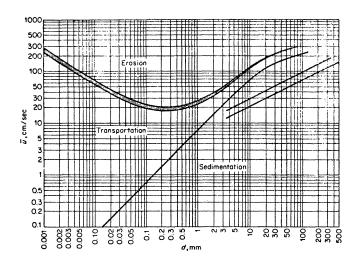
Fig. 1. Erosion-deposition criteria for uniform particles (After Hjulström, 1935)
