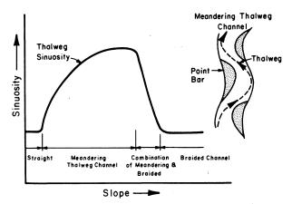
Fig. 2. Sinuosity vs. Slope with Constant Discharge. (Channel patterns are illustrated in Fig. 1.)
