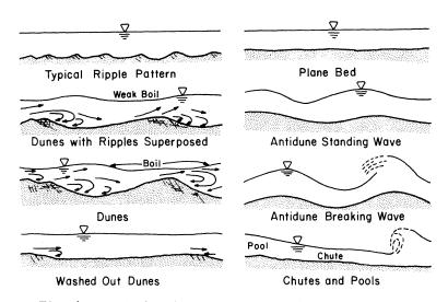
Fig. 6. Typical Bed Forms in Sand-bed Channels (Simons and Richardson, 1966)
