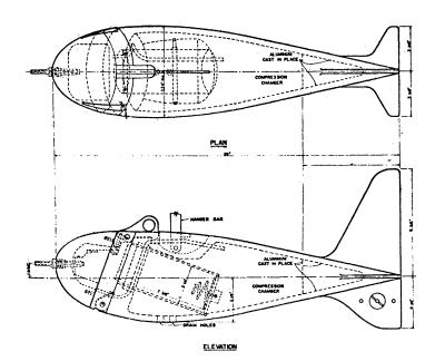
Fig. 11. US P-61 Point-integrating suspended-sediment sampler (Interagency Committee, 1963)
