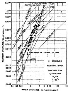
Fig. 3. Sediment discharge as function of water discharge for Niobrara River near Cody, Neb., obtained from observations and calculations by several formulas
