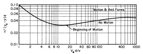
Fig. 5. Shields Relation for Beginning of Motion
