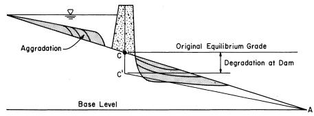
Fig. 10. Channel Adjustment Above and Below a Dam
