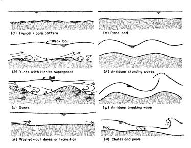
Fig. 4. Idealized bedforms in alluvial channels (After Simons et al., 1961)
