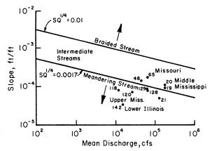
Fig. 3. Slope-discharge Relation for Braiding or Meandering in Sand Bed Streams (Lane, 1957)
