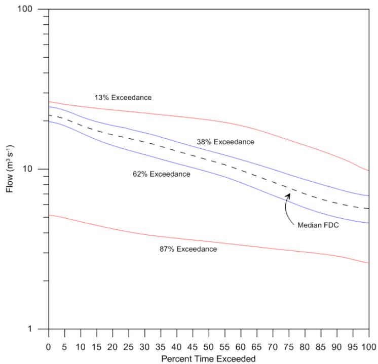
**Figure 4** A median FDC and associated levels of dispersion.
