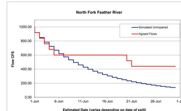
North Fork Feather River flows agreed to during license test flow period (2015-2020), compared to unimpaired gradual recession rate. Bench out at 600 cfs for 15 days is for recreational boating. Required for any spills after May 1.
