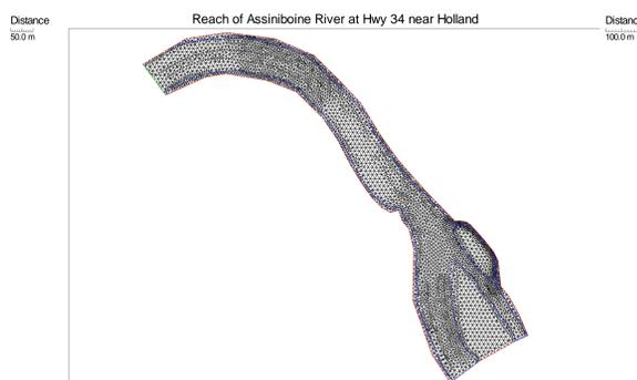
Figure 3 Finite element mesh generated for Reach 3, Assiniboine River at Hwy 34 near Holland
