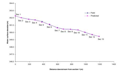
Figure 6 Comparison between the predicted and field water surface elevations for the calibration discharge at Reach 2, Assiniboine River at Brandon Riffles
