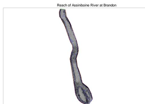
Figure 4 Finite element mesh generated for Reach 2, Assiniboine River at Brandon Riffles
