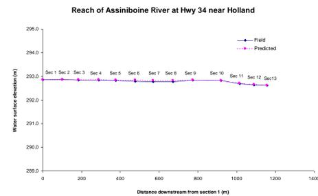
Figure 5 Comparison between the predicted and field water surface elevations for the calibration discharge at Reach 3, Assiniboine River at Hwy 34 near Holland
