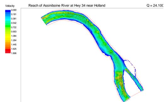
Figure 7 Predicted velocity contours along Reach 3, Assiniboine River at Hwy 34 near Holland (Q = 24.1 m<sup>3</sup>/s)
