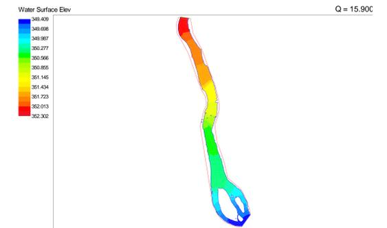
Figure 8 Predicted water surface contours along Reach 2, Assiniboine River at Brandon Riffles (Q = 15.9 m<sup>3</sup>/s)
