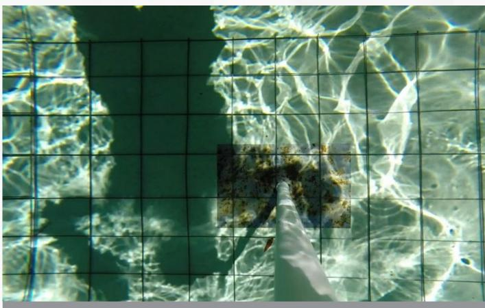
nrectified photo shows distortion of square calibration grid cells
