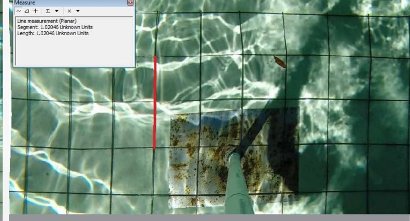
Rectified photo showing square grid cells
