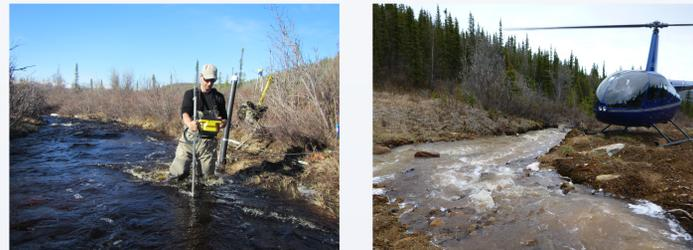
Access to streams at the site is almost entirely helicopter only. Flow measurements were taken at established PHABSIM transects using a Flo-Mate 2000.
