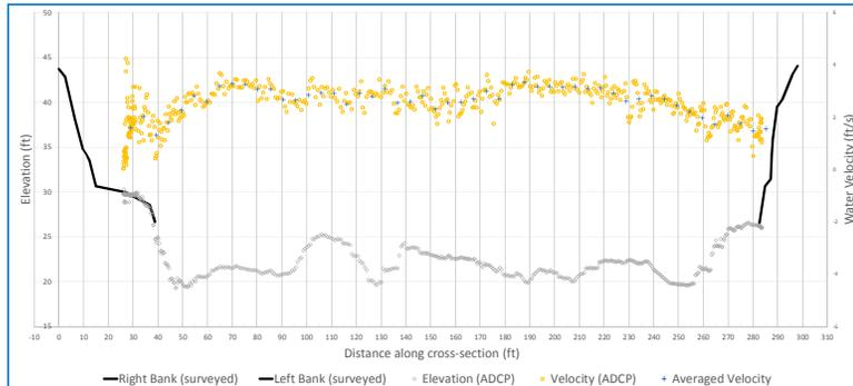
Figure 3. The shoal-type cross-section and velocity profile used for this study. Bank geometry (above waterline) was surveyed with a total station; bed elevations/depths were measured with ADCP and converted to NAVD. Mean water column velocities were measured with ADCP, then averaged over 5-ft intervals along the cross-section.
